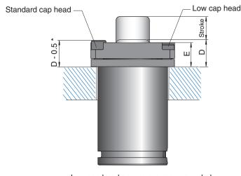
Low cap head screws are recommended \* If standard screws are used
